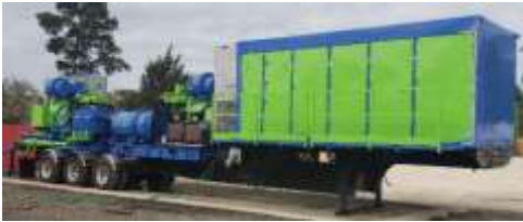
Electric Frac Unit (Lime)
